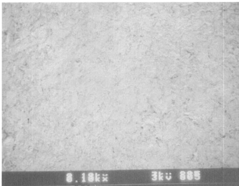
FIGURE 4a. SEM of an uncoated pellet surface dried by fluidised-bed methodology; magnification x400.
