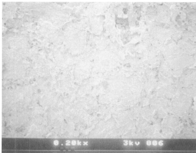
FIGURE 5a. SEM of an uncoated pellet surface dried by fluidised-bed methodology; magnification x800.
